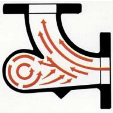
Figure 1: A cross section of the new type of elbow in use at Chromalloy. Suspended material coming from the right forms the slowly revolving soft mass of product suspended in air. The soft ball revolves slowly, and is self-renewing as some new product is added at the top and particles leaving the bottom deflect and join the main product stream.
